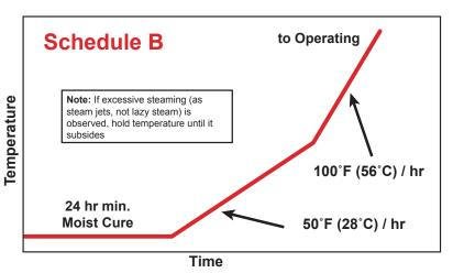
Moisture driven and entrapped in the back up insulation is dangerous and may lead to spalls/explosions at elevated furnace temperatures. This is of special concern in floors/hearths.
